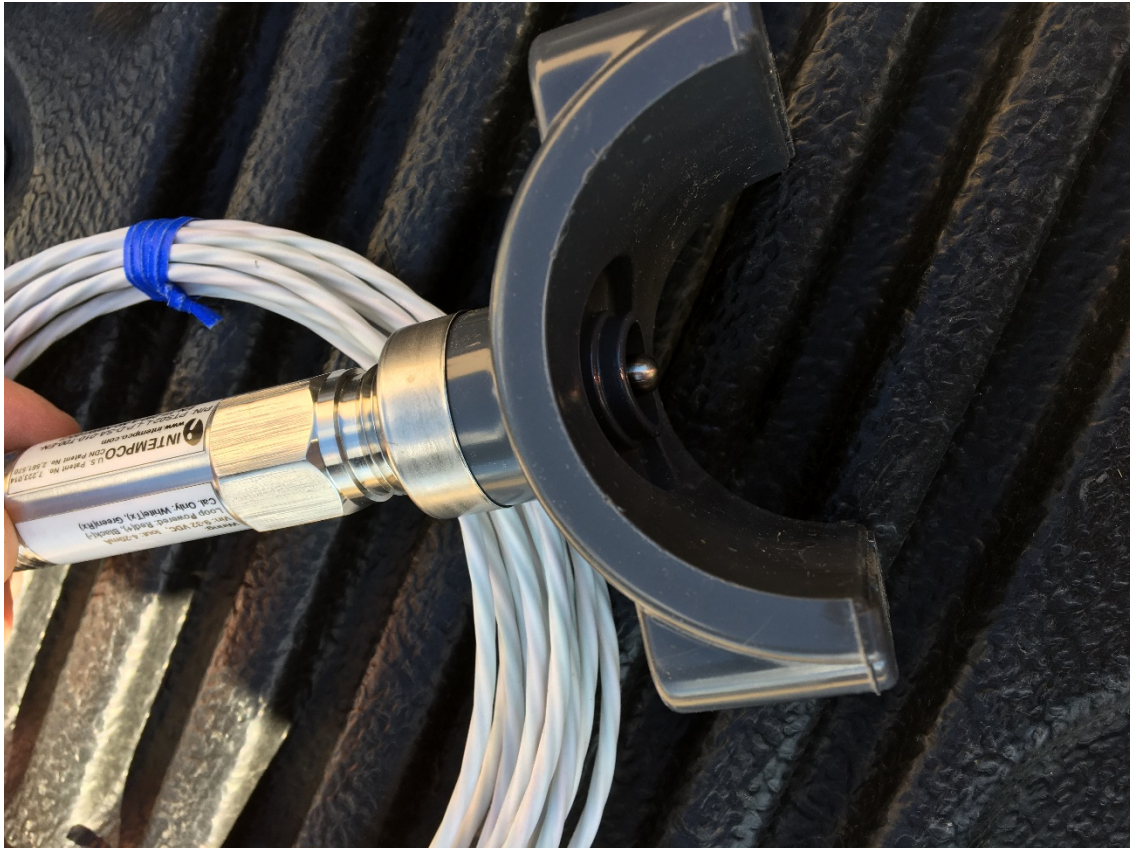
Figure 3. Wellhead Temperature Sensor and Adaptor Saddle
