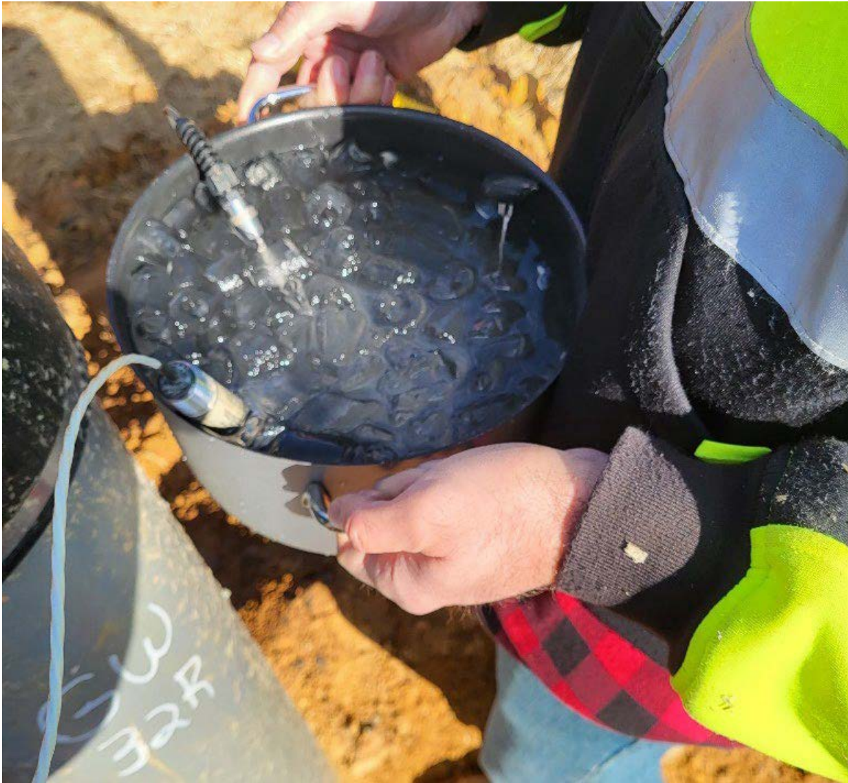
Figure 5. Testing Accuracy of Temperature Sensor using an Ice Bath
