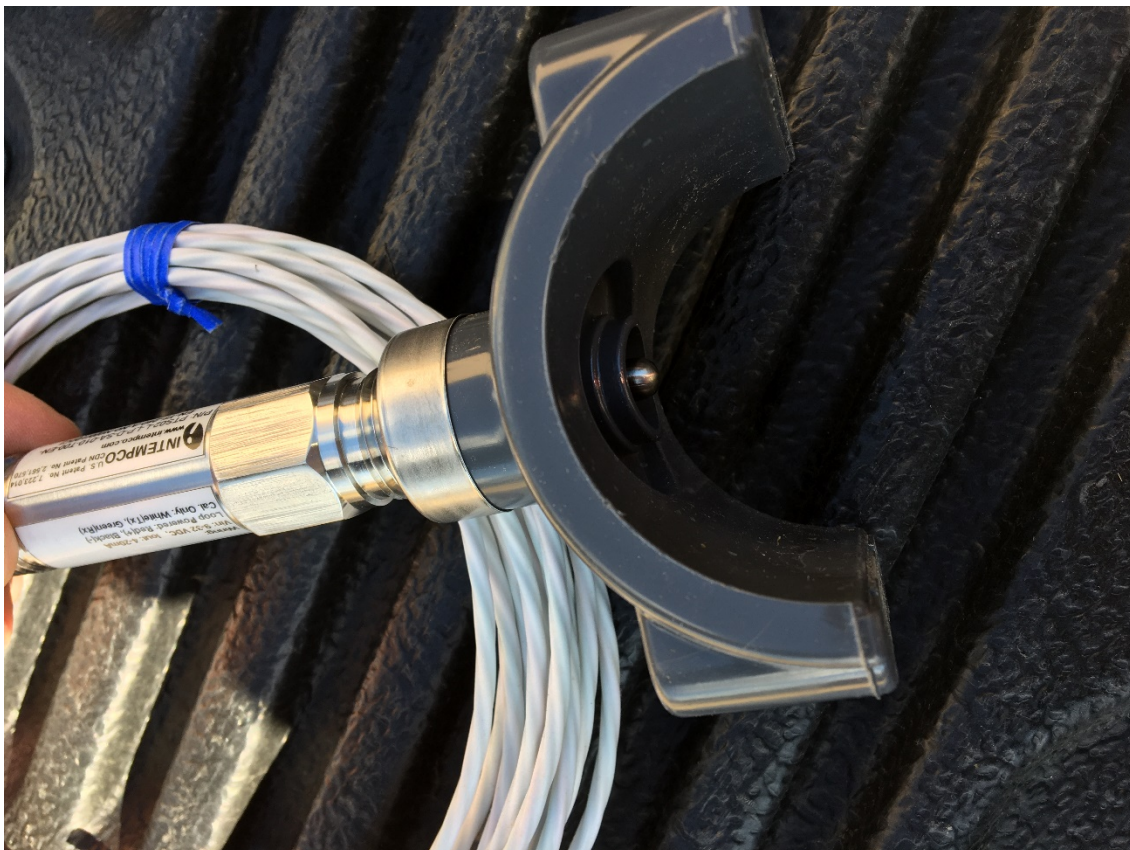
Figure 1. Wellhead Temperature Sensor and Adaptor Saddle
